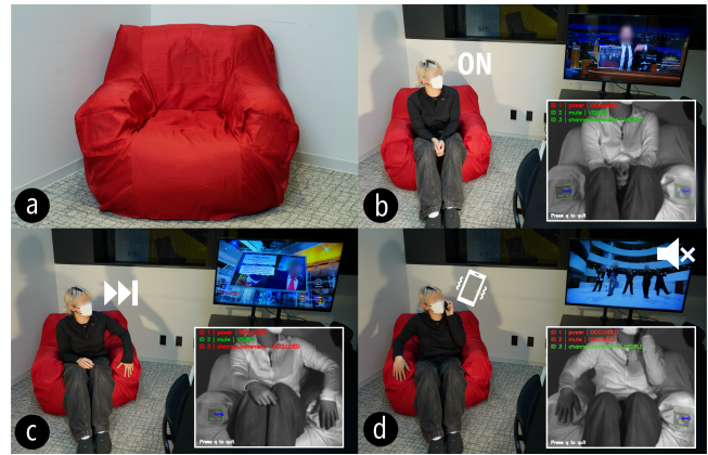
Figure 12: Sofa-integrated TV control using industrially woven markers.
