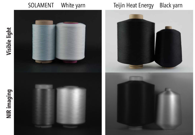
Figure 2: Visible-light and NIR images of SOLAMENT (8%) and Teijin Heat Energy yarns compared with normal white and black yarns, respectively.
